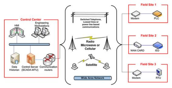
Figure 6. A general supervisory control and data acquisition (SCADA) architecture. HMI, human-to-machine interface; MTU, master terminal unit; PLC, programmable logic controller; IED, intelligent electronic device; RTU, remote terminal unit; WAN, wireless area network.
