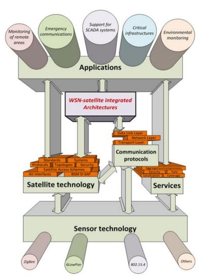
Figure 1. A taxonomy for the definition of wireless sensor network (WSN)–satellite architectures. SCADA, supervisory control and data acquisition; BSM SI-SAP, Broadband Satellite Multimedia Satellite Independent–Service Access Point.
