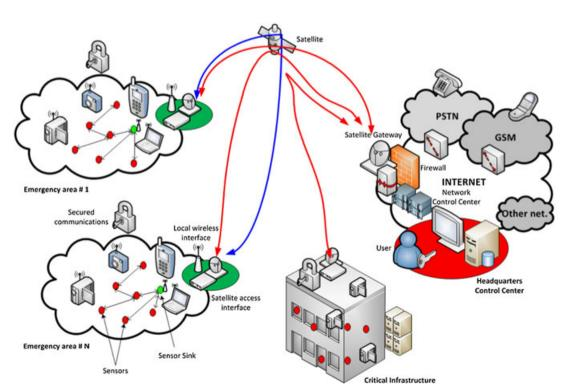
Figure 8. Architecture and network configuration for the emergency scenario. PSTN, public-switched telephone network; GSM, Global System for Mobile Communication.
