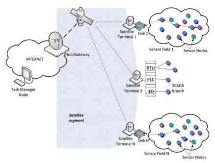
Figure 2. A generic satellite-based wireless sensor network architecture. RTU, remote terminal unit; PLC, programmable logic controller; IED, intelligent electronic device; SCADA, supervisory control and data acquisition.
