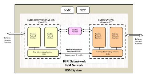
Figure 5. Broadband Satellite Multimedia (BSM) reference model. NMC, network management centre; NCC, network control centre; SI-SAP, Satellite Independent-Service Access Point.
