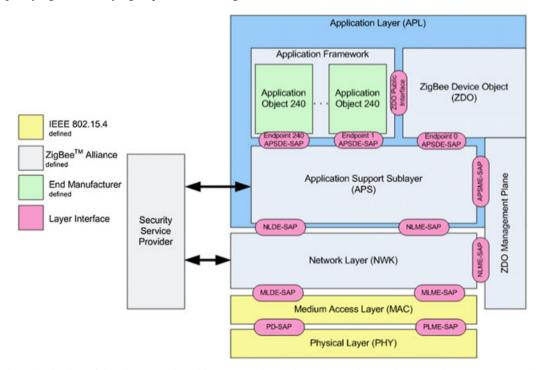
Figure 4. Outline of the ZigBee stack architecture. APS, sub-layer data entity (APSDE); APS Management Entity (APSME); Network Layer Data Entity (NLDE); Network Layer Management Entity (NLME); Mac Layer Data Entity (MLDE); Physical Data (PD); Physical Layer Management Entity (PLME).
