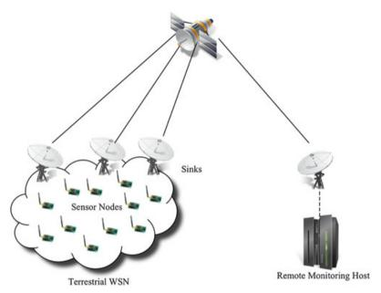
Figure 12. Architecture for environmental monitoring system. WSN, wireless sensor network.
